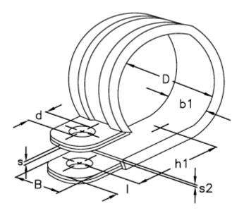
$\begin{array}{lll} \text{b1} & = 31.0 \\ \text{d} & = 10.5 \\ \text{Diameter D} = 24 \\ \text{h1} & = 29.5 \\ \text{I} & = 10.0 \\ \text{s} & = 1.00 \\ \text{s2} & = 3.0 \\ \text{Width B} & = 25 \\ \end{array}$
